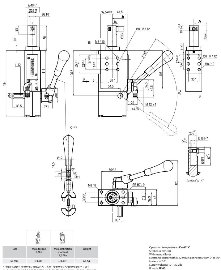
\* : TOLERANCE BETWEEN DOWELS ± 0,02, BETWEEN SCREW HOLES ± 0,1 \*\* : DIMENSIONS TO BE RESPECTED IN CASE OTHER MANUAL LEVERS ARE USED
