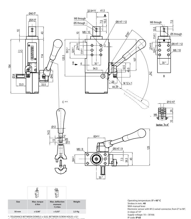
\* : TOLERANCE BETWEEN DOWELS ± 0,02, BETWEEN SCREW HOLES ± 0,1 \*\* : DIMENSIONS TO BE RESPECTED IN CASE OTHER MANUAL LEVERS ARE USED
