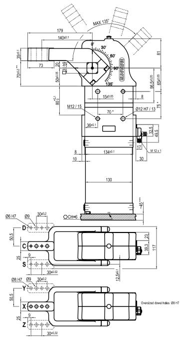
\* : TOLERANCE BETWEEN DOWELS  $\pm$  0,02, BETWEEN SCREW HOLES  $\pm$  0,1 \*\* : TOLERANCE AT 80 mm FROM PIVOT POINT \*\*\* : AREA TO ACCESS ANGLE ADJUSTMENT
