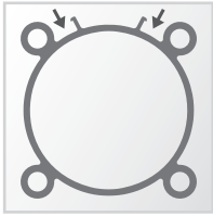
Tube profile with integrated sensor grooves UNIVER Original since 2005
