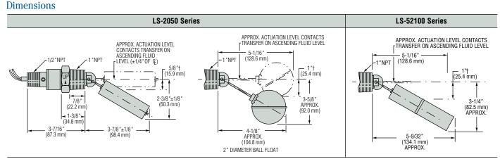
+Approximate de-actuation level, nominal (based on a liquid specific gravity of 1.0).
