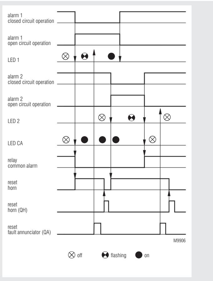
**Function Diagram (Common Alarm Annunciator Manual Reset)**
