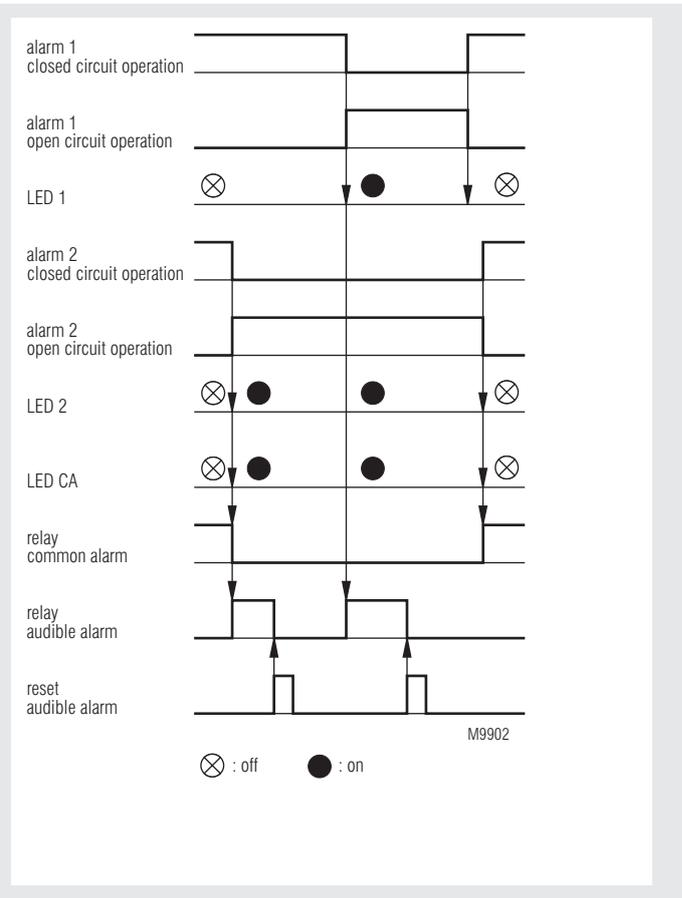
**Function Diagram (New Signal Alarm Annunciator)**
