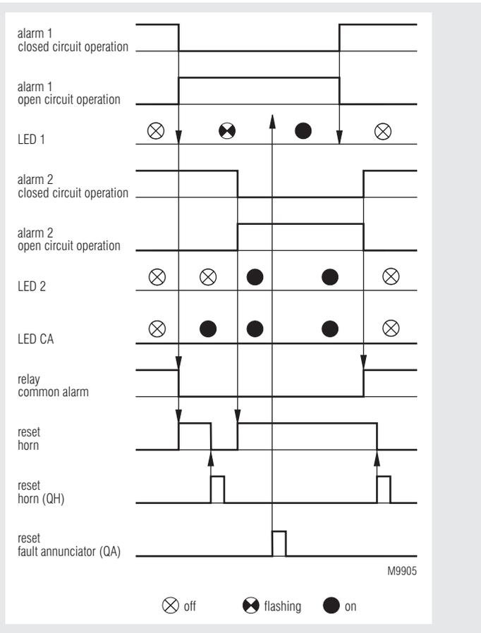
**Function Diagram (Common Alarm Annunciator, Auto Reset)**
