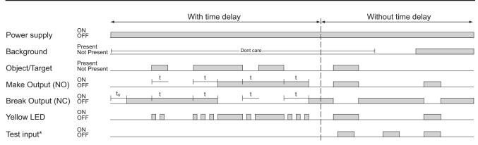
$t_v$  = Power on delay, t = Time delay (delay on operate and delay on release)
