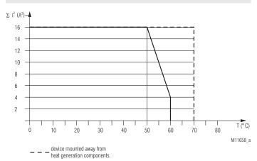
device mounted without distance heated by devices with same load.
