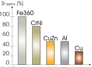
**Fig. 2** The rated operating distance is reduced by the use of metals and alloys other than Fe360. The most important reduction factors for inductive proximity sensors are shown in the figure.
