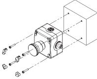
to access the holes. The wall fixing screws and the ones for closing the housing cover can be sealed with 4 caps (supplied with the housing). The caps not only give the housing a more pleasant look, but they also prevent the accumulation of dirt inside the recesses of the screws besides making tampering more difficult.
