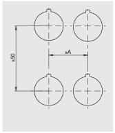
3-slot mounting adapter A=30 mm
