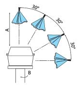
ISO 20653 envisages a particularly strenuous test. This test simulates the conditions of pressure washing in industrial environments with water jets having pressure between 80 and 100 bar, flow rate between 14 and 16 l/min. and a temperature of 80°C.
