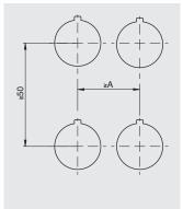
3-slot mounting adapter A=30 mm
