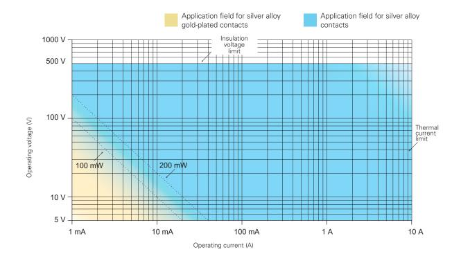
100 mW Recommended limit for general applications with snap action contact blocks with silver alloy contacts.200 mW Recommended limit for general applications with slow action contact blocks with silver alloy contacts.
