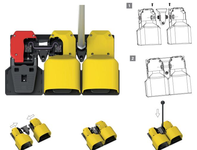
Besides the possibility of joining from two to four single foot switches, the joining elements make it possible to apply a metal tube that enables the electrical connection between the foot contacts and the contacts of an emergency push button, connected to the same tube, preserving thus an IP65 protection degree.
