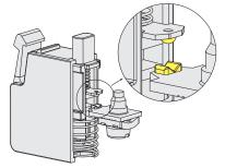
"V-shape" self-cleaning contacts with guadruple support point. This type of shape, thanks to the presence of the double support point, makes it possible to drastically reduce the probability of contact commutation failure. In addition to this, it improves considerably the reliability in the presence of dust.
