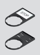
Label holders for single device, adjustable by 90° in 90° increments. The switch labels of other manufacturers can be used (for example: 3M article KE-7270-2691-3 or GRAFOPLAST article SITM612X) as long as they have the following dimensions: base 27 +0/-0.4 mm, height 18+0/-0.4 mm, thickness 0.8  $\pm$ 0.4 mm.
