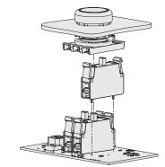
Versions with panel mounting of the EROUND series contact blocks with solder pin are available. If there is no wiring but a printed circuit, these contact blocks can be directly welded on the latter.
