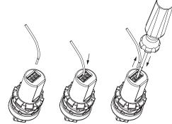
The potentiometer is provided with a three-pole terminal board with PUSH-IN type spring-operated connection. This technology allows a very handy quick wiring procedure. The wire is simply inserted into the appropriate hole, without the need for any auxiliary tooling, through the use of rigid or flexible wires with crimped wire-end sleeve. Release is obtained by pressing the appropriate wire-releasing button.
