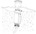
Protected contact block for control devices fitted in switching cabinets with the presence of dust also inside the cabinet. The block ensures an IP67 protection degree for internal electric contacts.
