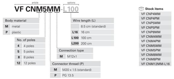
ATTENTION: always disconnect the power supply before removing the connector. The connector is not suitable for separation of electrical loads. Note: the 12-pole connector is only available in metal with M20x1.5 thread and 16 cm wires.
