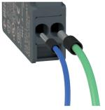
The PUSH-IN spring connection allows quick and simple wiring, as the wire just needs to be inserted into the appropriate hole in order to establish the electrical connection and automatically secure the wire. The reduced force required to insert the wire allows completely toolfree connection by using wires with crimped wire-end sleeves. They are released by pressing a special wire release button - including individually - with any tool, without the need to use a screwdriver of a predefined size.
