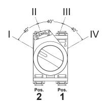
Note: The LED supplied with the illuminated selector switch has a supply voltage of 12 ... 30 Vac/dc. Other voltages on request.
